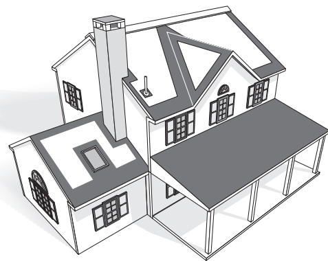
Figure 7-6: The dark shaded areas are the places that WinterGuard helps protect from the melting water coming off the ice dam.
