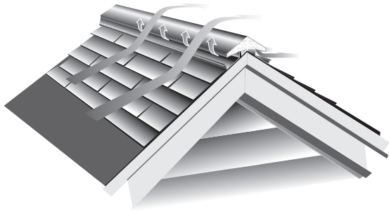
Figure 7-20: A bafled FilterVent® creates an area of low pressure on both sides of the ridge vent. It literally lifts air out of the attic through both sides of the vent.
